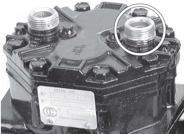
Stripped Fitting due to overtightening service valve.
