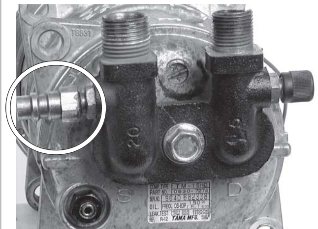
Retro-fitted to 134a, system not flushed.
