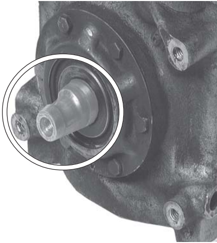
Keyway not properly installed on compressor shaft.
