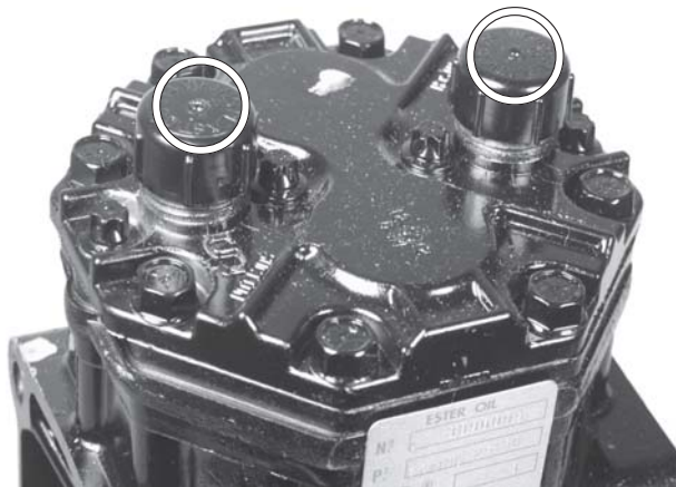
Oil leaking from center of shipping cap. Factory nitrogen charge may cause slight oil leak from center of cap while in box. Check oil level prior to installing compressor.
